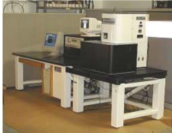
Model 770 Scanning SQUID Microscope with dc and ac biasing magnets
