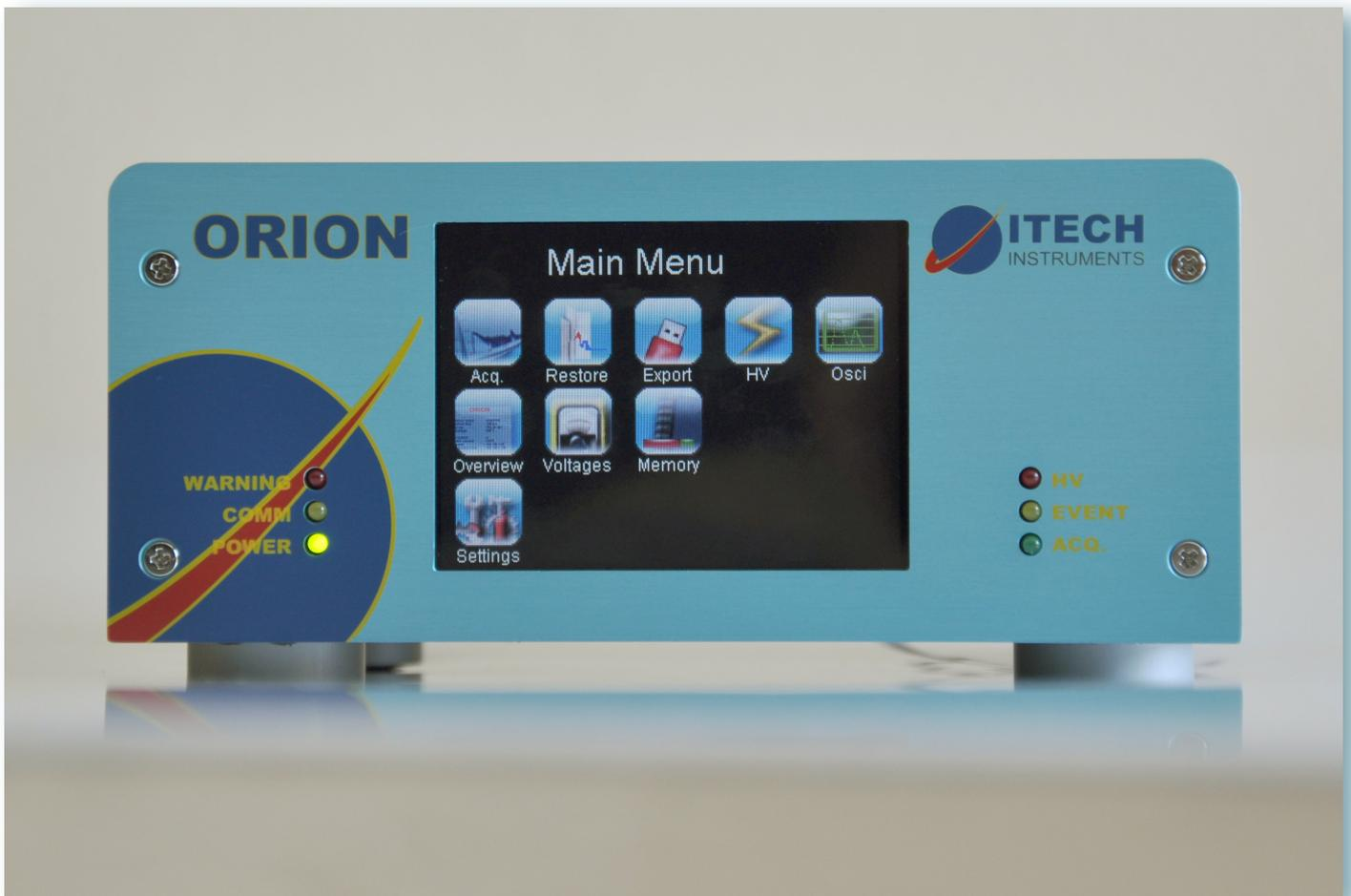
The **ORION** is the most advanced digital signal processor developed by ITECH INSTRUMENTS. It is a 64K channel analyzer based with 100% digital signal processing. The **ORION** features a 100 MHz 16 bit sampling ADC, an internal Linux computer, and internal high voltage bias supply all supporting pulse height analysis, list and peak shape data acquisition.
