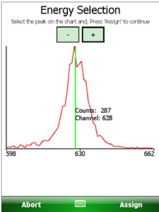
6) Use the + and – buttons to zoom in/out on the peak of interest. The peak can be centred on the screen by dragging with the stylus to the right or left.
