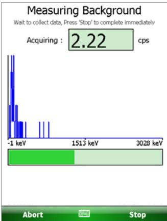
2) While the background is being measured the green bar at the bottom shows the progress.
