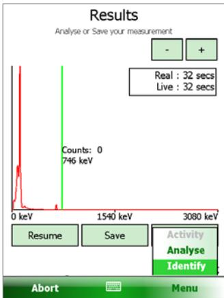
2) Press "Menu" on the bottom green bar to display the analysis options. Pressing 'Identify' runs the ID algorithm on the collected data.
