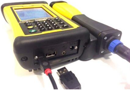
Connect the RayMon to the computer running **MultiSpect Analysis** using a mini USB 2.0 cable.
