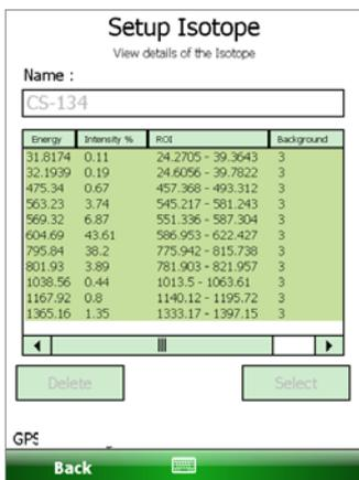
8) If an isotope is required that is not in the built in library, it can be added manually. On the Category Setup screen press “Create”. This leads to the Setup ROI screen.
