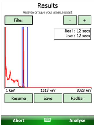
6) Pressing "Back" again displays the graph with the energies displayed in the results table identified by blue lines on the graph.
