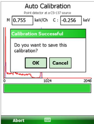
2) After the acquisition has completed the operator will be given the option to use the calibrated values.
