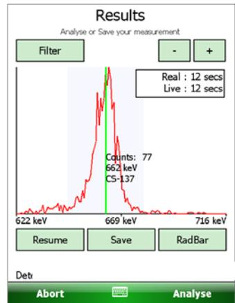
6) The green cursor can be used to measure the counts in a specific channel. Use the stylus to move the cursor position.
