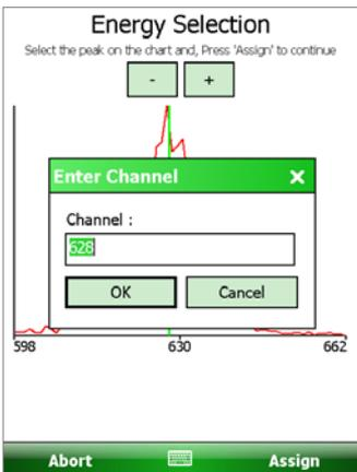
8) The channel number for the cursor position will be displayed. If this is in the correct place select “OK”. If not, adjust the value until the centroid is found.
