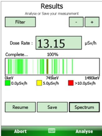
7) If RadBar has been enabled in the measurement settings, pressing the 'RadBar' button will display the RadBar of the measurement and the total dose rate measured. The RadBar can be zoomed and scrolled in the same way as the graphs. To return to the spectrum press the 'Spectrum' button.
