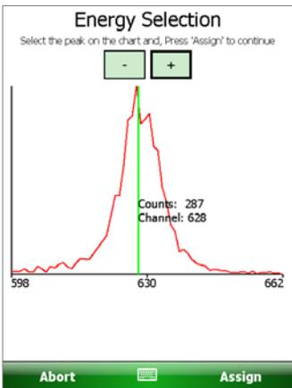
7) Place the green cursor line on the centroid of the peak relating to the source and press “Assign”.
