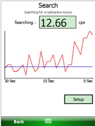
2) Search mode works by comparing the measured total counts from the detector in a fast response channel (red line) to a background level (blue line).
