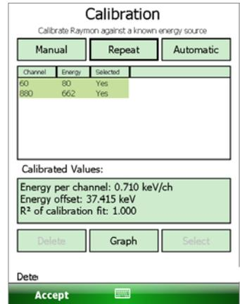
11) Pressing “Graph” displays a graph of the calibration points and the straight line fit. This graph is useful for identifying errors in the calibration points.
