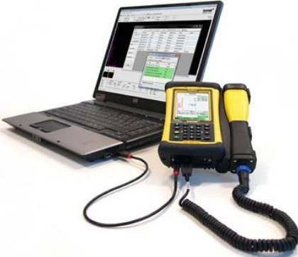
From within **MultiSpect Analysis** navigate to your measurements database and use the “import from device” functions.
