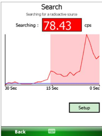
If the measured counts exceed the background level by a significant amount, the user is alerted to the presence of a radiation source by the count rate box becoming red and the graph being given a red shading.
