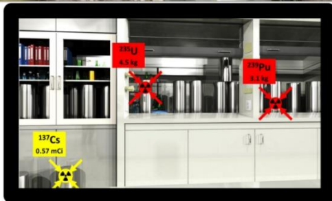
Figure 1. CBRNE team members analyze the radiological situation upon entering a nuclear weapons production site. The visual nuclear threat information from the imaging detector shows the identities, locations and quantities of the radiological materials on an intuitive visual display.
