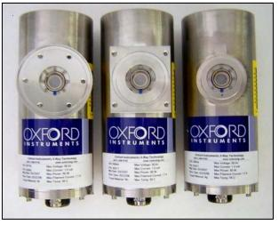
The package can be supplied with a high voltage well connector and a triax connector for the filament supply. The tube is to be operated in a positive anode mode with the cathode grounded. The standard exit window is 0.005 inch Beryllium.
